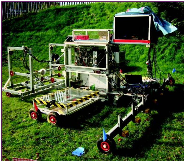
The Mapping the Underworld Mobile Laboratory, with Passive Magnetic Field, GPR and Vibro-Acoustic Sensors (looking from left to right).
