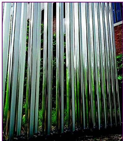
Prototype Sonic Crystal based noise barrier developed at Loughborough University.
